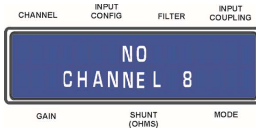
Figure 2.5 – Missing or Defective Card
