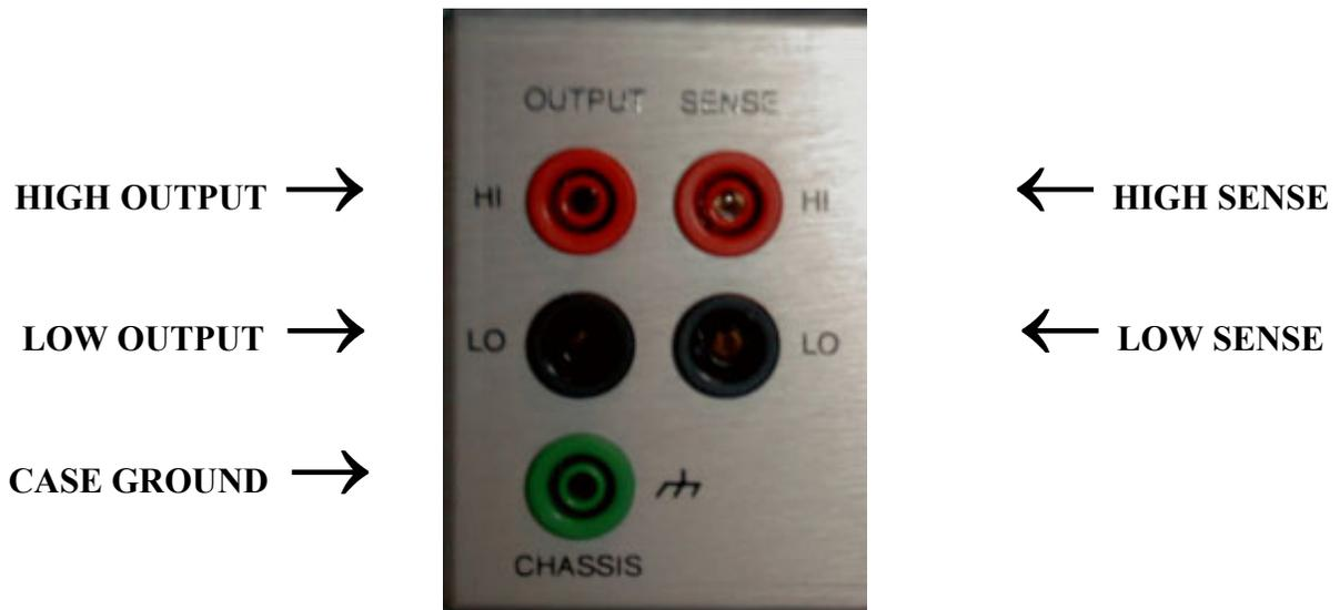
*Figure 2.6 Optional Rear Output Terminals*
